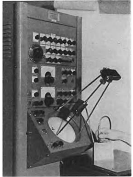
FIG. 2c. Fixed focus camera which is quickly attached for recording reflectograms when desired, although visual observation of the oscilloscope screen is the usual practice.
